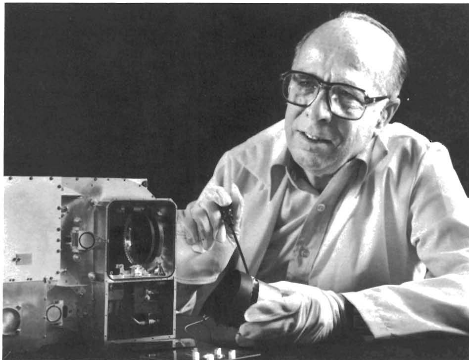
Fig. 9. Equipment carried by ISEE-3 for the Los Alamos plasma experiment. The instrument has a 135-degree spherical-section electrostatic analyzer (behind the upper opening) followed by a secondary emitter system (the concave disk in the upper opening) and a 20-stage focused mesh electron multiplier (held by Samuel Bame). The number of electrons in each of fifteen contiguous energy bins from 8.5 eV to 1.14 keV is counted by varying the voltage stepwise on the analyzer plates. From these data the density, flow speed, temperature, and heat flux of plasma electrons everywhere along the spacecraft's orbit can be determined.
